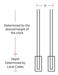
The following information for installing the mounting poles/ beams are suggestions only. Local codes, field placement, customer preference, and other special considerations will determine the specifics of your installation, including footer specifications, above ground height, and total length of the poles/I-beams.
