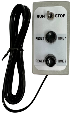
(1) Handheld Shot Clock Controller Connects directly to the LCD controller
